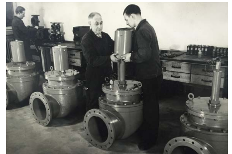
In 1961, special valves derived from the old 1000 series were produced for Hamburg's main post office's pneumatic delivery system.
