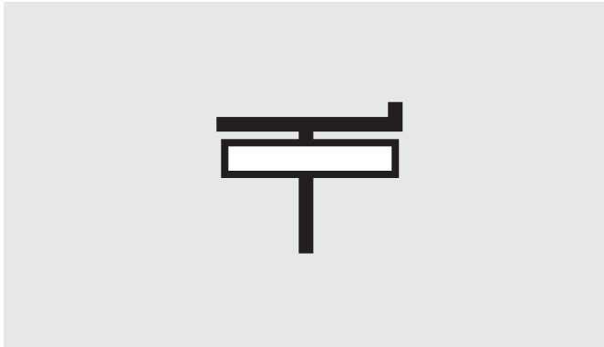
Manual operator "Manually operated via gearbox or servo"
